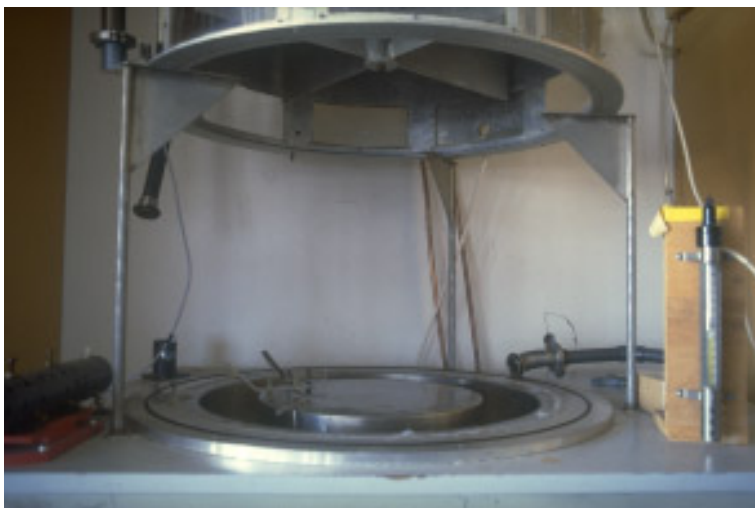
Figure 1: Detail view of the small circular facility at Heidelberg University. The cover with the wind paddle has been lifted to give view to the annular water channel with a cross section of 10 \times 10 \text{ cm}^2 . (For color figure, see Plate 18.)
