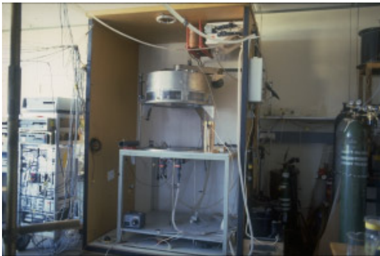
Figure 2: The small circular wind-wave facility at Heidelberg University was contained in a thermostated box to run experiments between 4–35° C. The air space of the facility could be flushed with nitrogen at rates up to 60 l/min by evaporating liquid nitrogen from a tank with an electric heater (situated to the right of the thermostated box). (For color figure, see Plate 19.)
