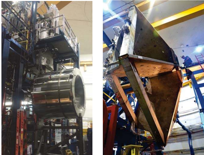
Figure 4: The CLAS12 magnet systems. Left: The fully assembled solenoid magnet including all cryogenic connections on the beamline at the beginning of cool down, before the detector installation. Right: The torus magnet with all six coils mechanically assembled in a common cryostat. The coil cryostat, which is fabricated from non-magnetic steel, has an outside width of 124 mm. The cross bars provide a cold (4.5 K) cryogenic connection of neighboring coils, and counteract the out-of-plane forces to provide mechanical stability to the full magnet. Due to the large physical size of the assembled torus magnet, the final assembly of the magnet had to be completed in Hall B.
