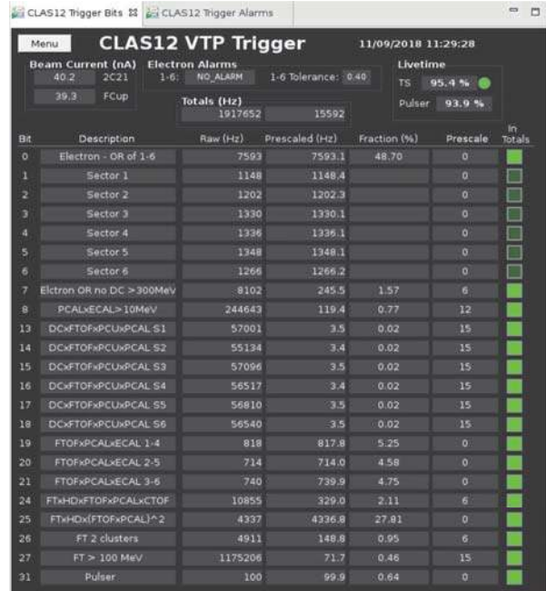
Figure 36: The CLAS12 trigger control screen during a specific data run with a total of 17 active triggers operating at a livetime of 95.4%. Nearly half (48.7%) of all triggers are from single electrons detected in one of the 6 FD sectors. Over a quarter (27.81%) of all triggers required an electron in the FT with an additional two charged hits detected in the FTOF and in the PCAL. Several others were taking data at the 5% level and required charged tracks in the FTOF and ECAL in opposite FD sectors. Finally, several other triggers were used for monitoring purposes and were heavily pre-scaled.
