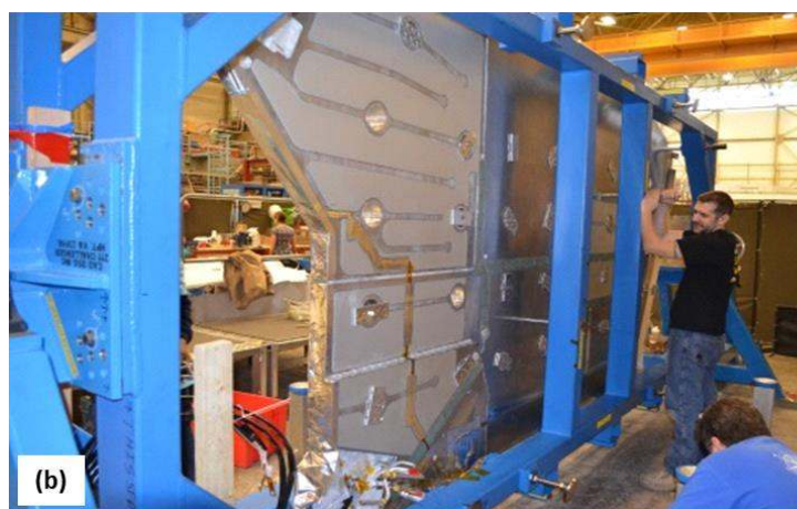
Figure 31: (a) Applying Multi-Layer Insulation (MLI) to coil case, (b) coil with thermal shield installed and in rotatable jig (to allow fitting of instrumentation on the other side).
