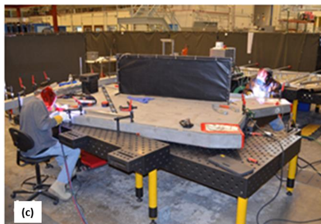
Figure 32: (a) Soldering additional copper stabilizer to the leads as they exit from the vacuum jacket, (b) Stabilized leads bent to required shape and insulated – ready for transport to the hall, (c) Welding shut the vacuum jacket.
