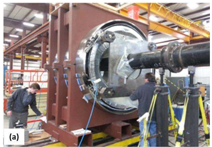
Figure 35: (a) Coil leads being routed on the outside of Coils 3 and 4, (b) Additional copper stabilizer being soldered to leads.
