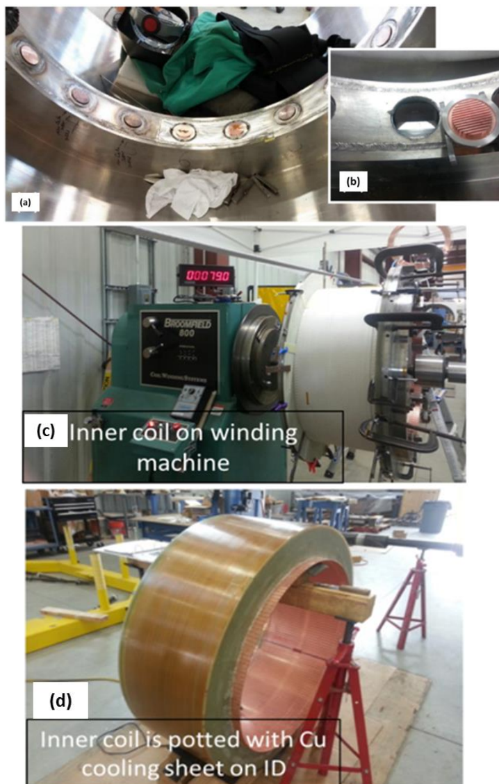
Figure 33: (a) Central cooling channel with helium “buttons” installed – the copper cooling sheet fingers were later soldered to these buttons, (b) Inset picture showing a helium button before welding into channel (the “fins” on the button face the inside of the channel), (c) One of the two inner coils being wound, (d) One of the two inner coils after epoxy potting was completed (the slotted copper cooling sheet can be seen on the inner surface of the coil, potted in with the coil).
