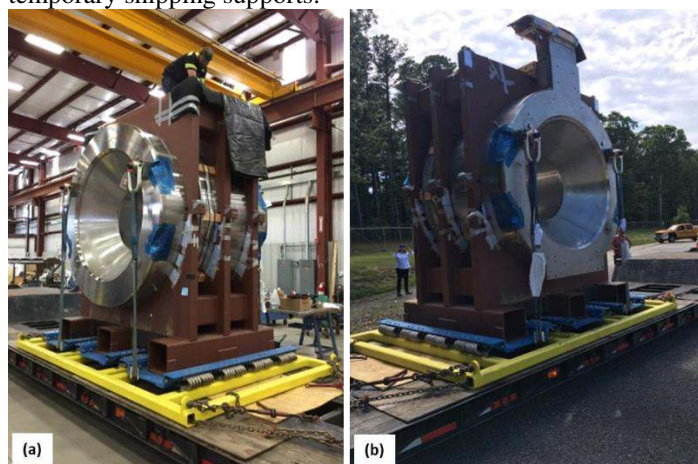
Figure 48: (a) Solenoid in shipping cradle and transport fixture at vendor, (b) Solenoid arrival in at JLab.
