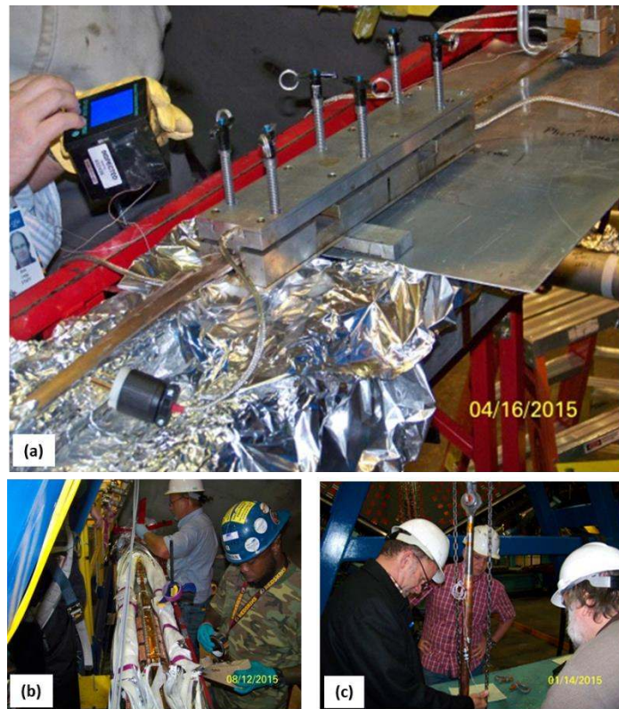
Figure 41: (a) Splice soldering using purpose-built temperature-controlled heating rig, (b) Applying MLI to the splice joints, (c) Load testing an axial support.
