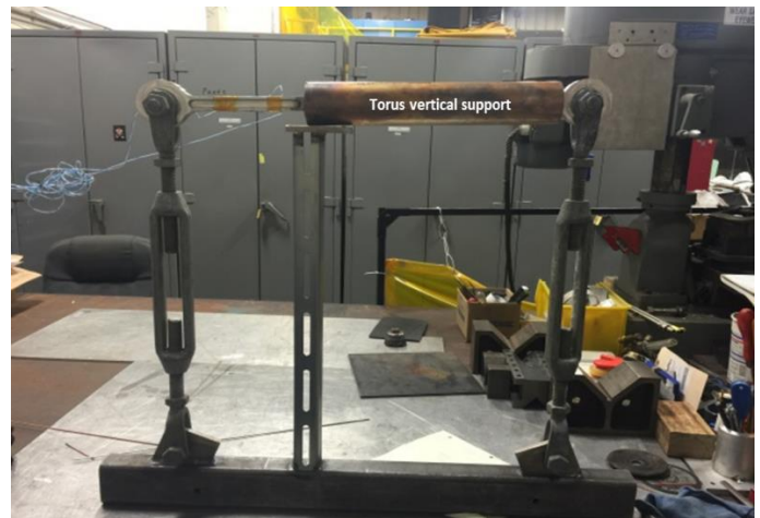
Figure 52: (a) Bend testing a spare torus vertical support.
