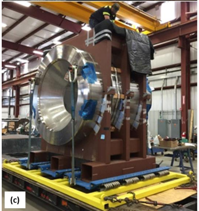
Figure 36: (a) Stycast being painted onto the outer diameter of Coil 5 after epoxy potting before being overwrapped with additional glass fiber cloth tape, (b) Inserting Coils 1-4 into the Coil 5 bobbin, (c) All five coils assembled together.
