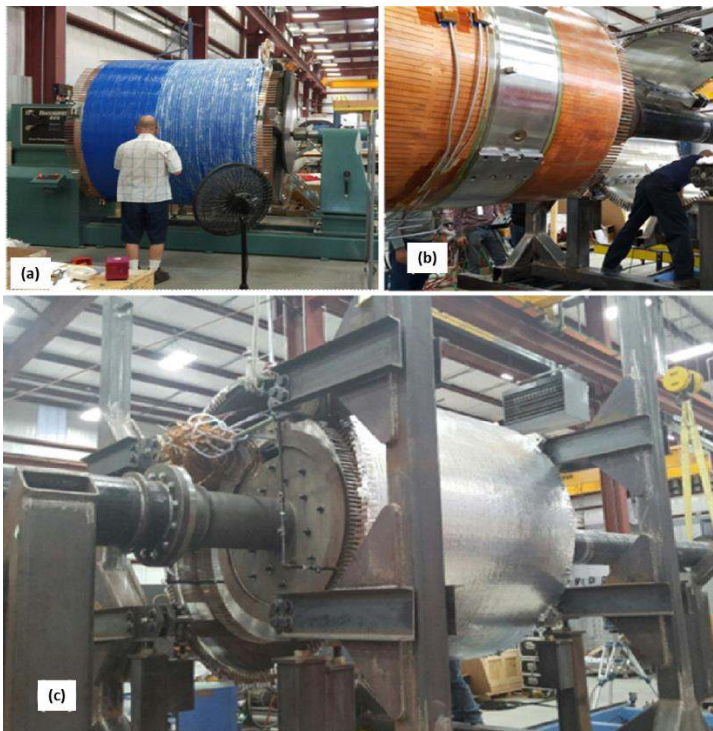
Figure 36: (a) Stycast being painted onto the outer diameter of Coil 5 after epoxy potting before being overwrapped with additional glass fiber cloth tape, (b) Inserting Coils 1-4 into the Coil 5 bobbin, (c) All five coils assembled together.
