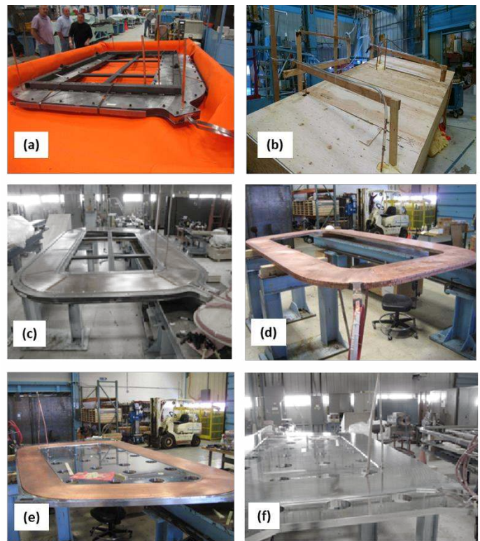
Figure 28: (a) Potting mold closed up ready for potting, (b) Hot box with potting mold installed, magnet leads, and fill/vent tubes penetrating. The box is sloped for bottom fill, (c) Top cover removed from potting mold after coil potting, (d) Coil removed from mold and flipped, cleaned up, and ready for cooling sheet attachment, (e) Coil aligned in coil case, (f) Coil case cover installed over the coil.
