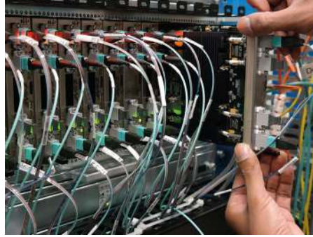
Figure 2. The overall upgraded trigger infrastructure. The 3 \mu TCA crates of the Layer-1 equipped with CTP7 boards (left) and the Layer-2 MP7 boards housed in a single crate (top).
