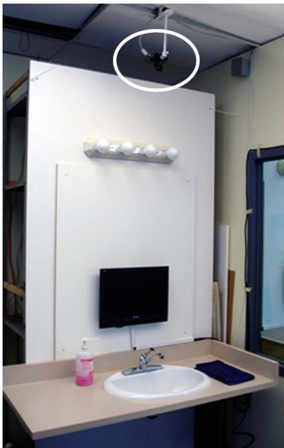
Figure 3 Example of the COACH system setup. (a) Example of the LCD screen, speakers (top-right), and video camera (circled) setup. (b) Example of a video-based prompt demonstrating how to turn on the water.
