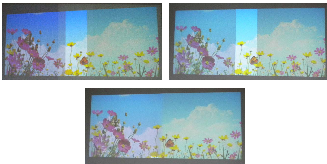
Figure 7. The left is the projected image before the color calibration and alpha blending; The right is the projected image after the color calibration but before alpha blending; The below is the projected image after the color calibration and alpha blending.
