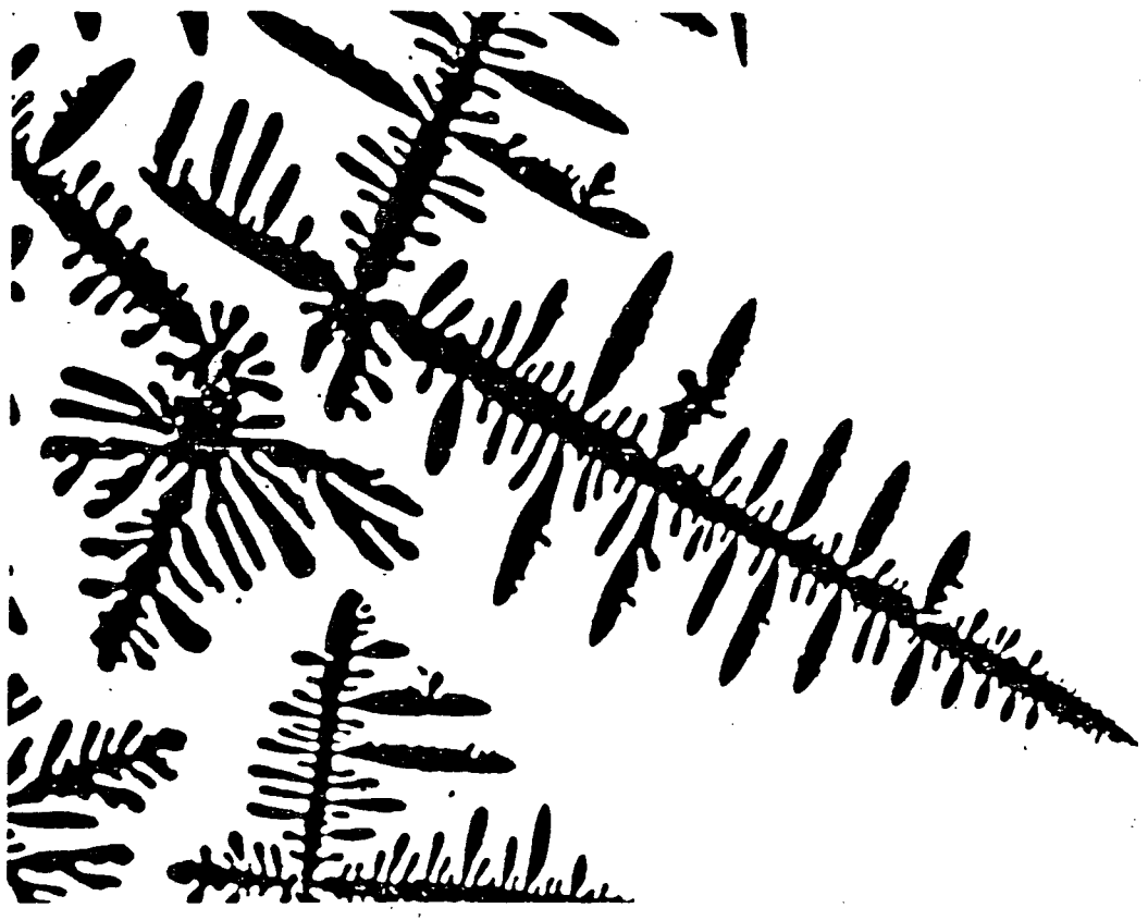
Figure 4 - Necking at the junction between the primary and the secondary dendrite and the secondary and the tertiary dendrite
