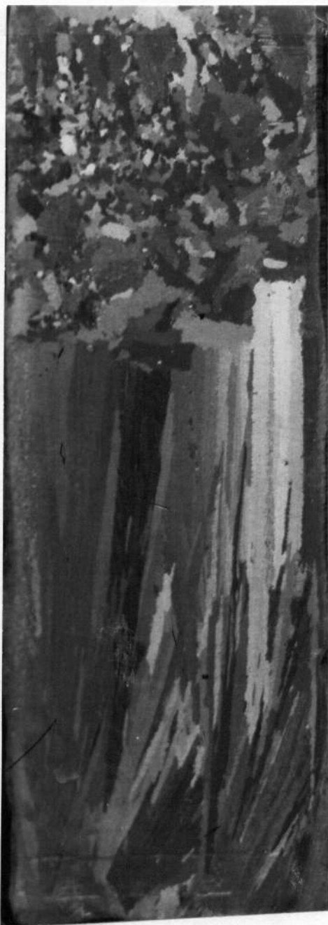
Figure 27 - Photograph of the sample cast with Fe powder addition in melt. Mag 1.8X.
