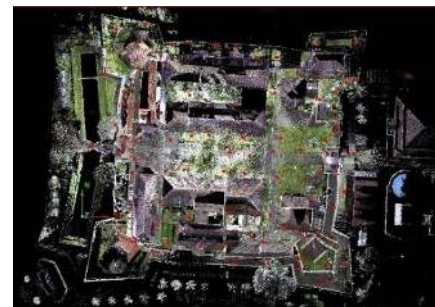
Figure 5. Terrestrial Lidar's scan station at Kotagede Great Mosque Building (a) and Vredenburg Fort Museum (b). Red circle denotes TLS scan station
