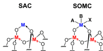
Scheme 1. Link between Single Atom Catalysts (SAC) on Oxide and Catalysts Prepared by SOMC on Oxides a
