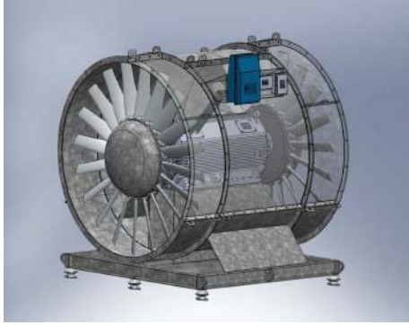
FIGURE 7: A computer-aided design model of the horizontal 2.8 metre two-stage double ended motor fan designed for the Marmaray project.
