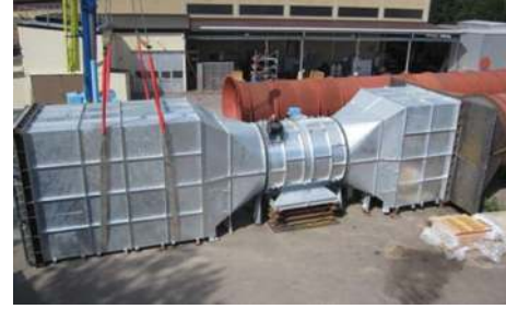
FIGURE 11: The first production Marmaray 2.8 metre two-stage double ended motor fan, transform, silencer, and damper package set up prior to its aerodynamic and acoustic test.
