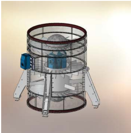
FIGURE 8: A computer-aided design model of the vertical 2.8 metre two-stage double ended motor fan designed for the Marmaray project.
