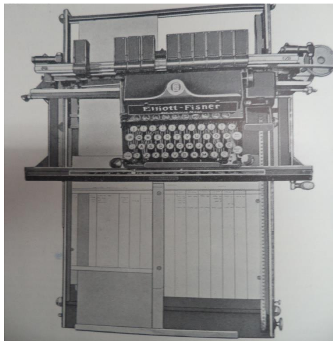
Figure 19 An Elliott-Fisher ledger posting machine (Foster 1929, 122)
