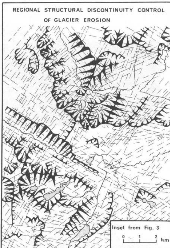
Fig.4. Primary fractures in the Snowdon (SW) and Glyder (NE) groups and principal glacier-eroded cirques and troughs. Fractures are shown by broken lines, cliffs by toothed shading, and lakes by stippling.
