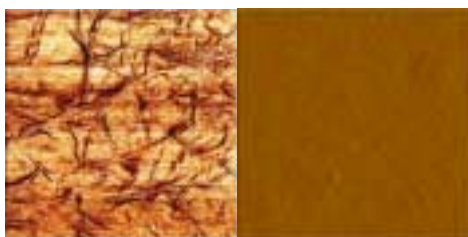
Figure 39. AFM phase images of a MEH-PPV/PF film containing 17% (left) and 4% (right) of MEH-PPV. Both scans are 3 \mu\text{m} \times 3 \mu\text{m} . The contrast covers phase angle variation in the 50^\circ range.
