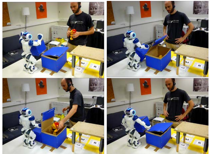
Figure 4. Shared plan execution. Left column: Human takes toy, Nao opens box, human places toy in box. Right column: Nao closes box.
