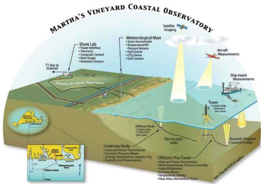
FIG. 3. A schematic representation of the MVCO showing the location of the meteorological mast, sea node, and ASIT. The cutout shows the actual location of these elements on the south shore of Martha's Vineyard.
