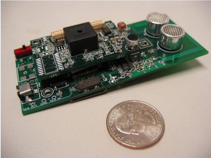
Figure 1-2: A Cricket node with a sensor board attached to it.
