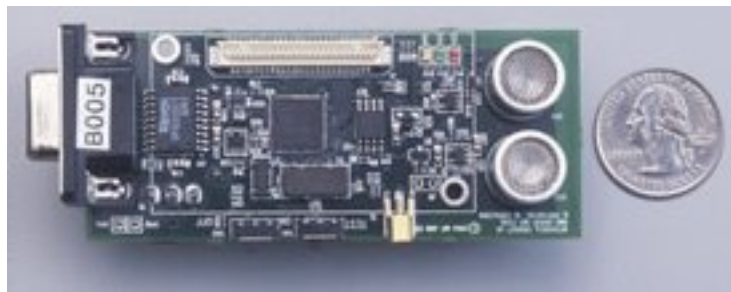
Figure 1-4: A Cricket hardware unit; this unit can function as either a beacon or a listener.
