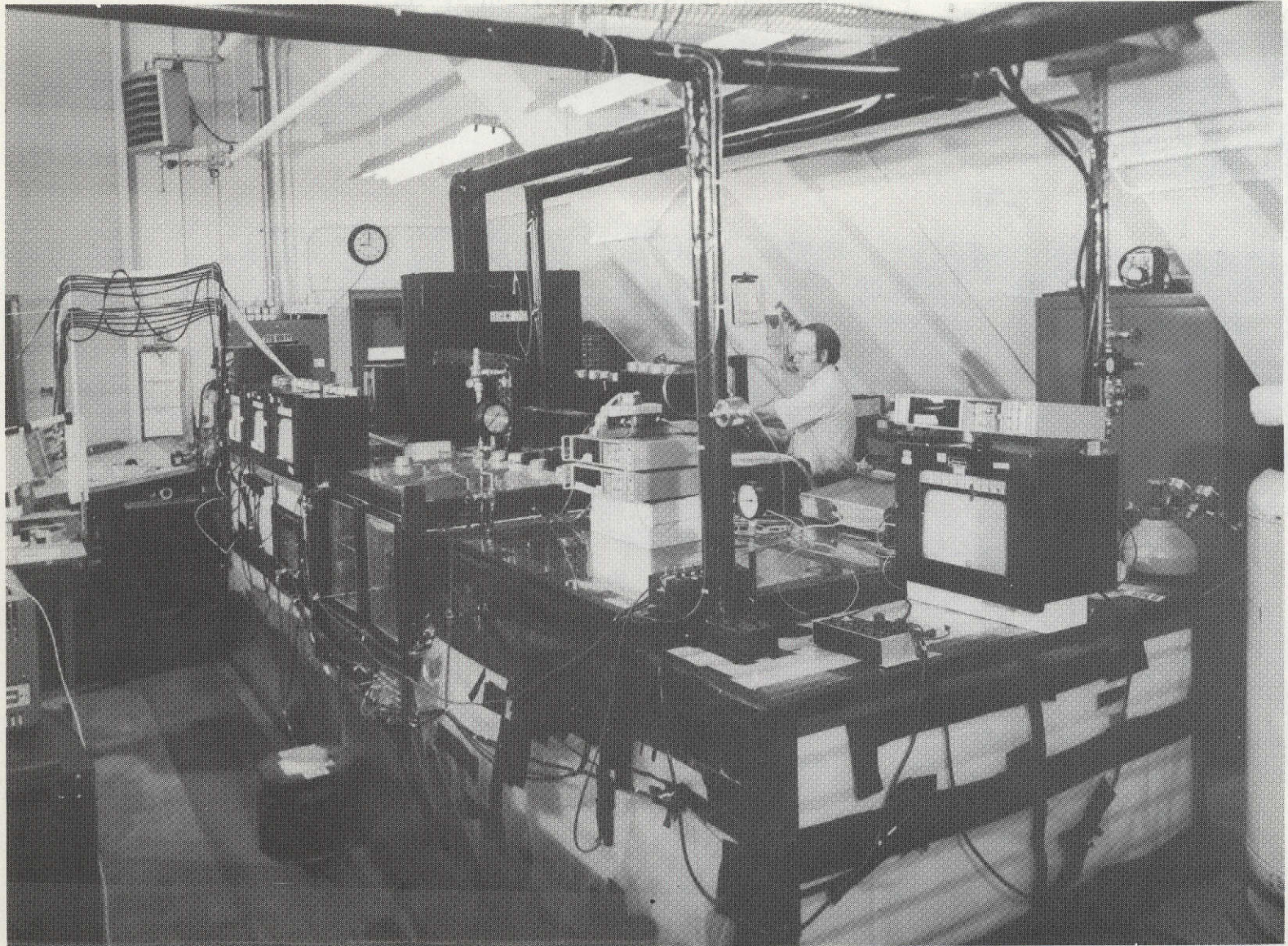
Figure 11.- Insulated low-speed tunnel and test apparatus.
