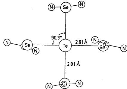
Fig. 1. The tetrakis(selenourea)tellurium(II) ion in the dichloride salt, as seen normal to the  $\text{TeSe}_4$  plane.
