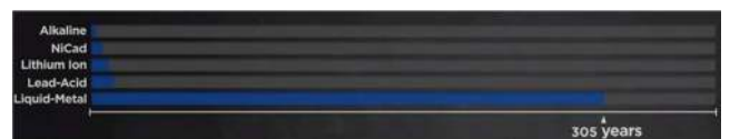
Fig. 14. The daily cycling of number of batteries showing liquid metal battery is capable of maintaining 80% of its initial efficiency during 305 years 'period [20].
