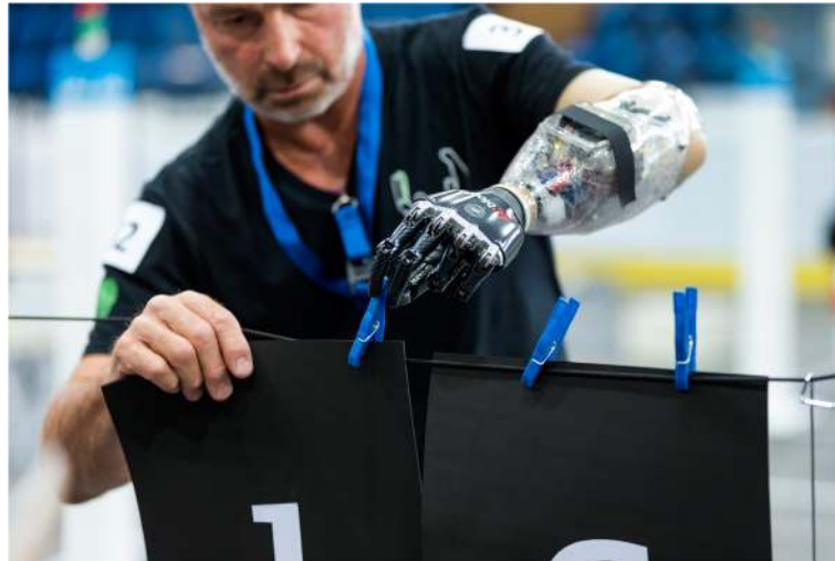
Fig. 2 Pilot with a powered arm prosthesis performing a daily living task. Picture was taken at the Cybathlon rehearsal in July 2015 by Alessandro Della Bella, ETH Zurich. The pilot on this image as consented to the publication of this image
