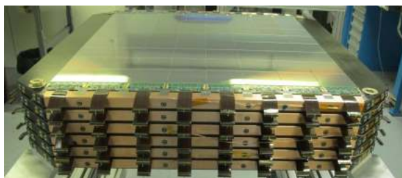
Figure 5: The STK before the assembly of the last tray. The 64 silicon detectors are visible, together with the horizontal copper bands used for the heat transfer.
