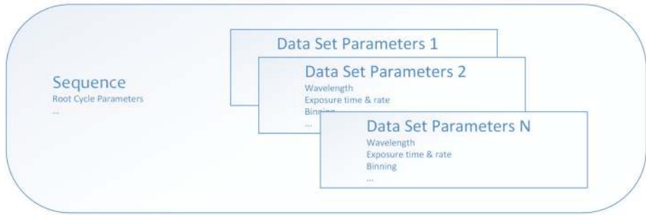
Figure 5 How DKIST instrument data acquisition, in particular also the VBI's, is programmed. Data set parameters (DSPs) encode the minimal set of settings required to acquire a particular data product, e.g. a number of images at a particular wavelength. Multiple DSPs can be sequenced through, guided by further parameters.
