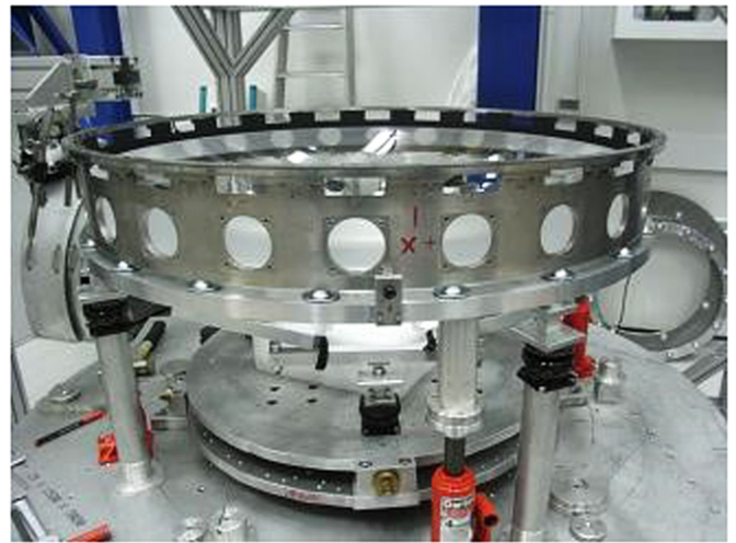
Figure 14. C1 lens partially installed in the C1 cell. The lens is supported from underneath on tip and tilt stages that are mounted on a rotary table. The cell is supported on jacks and its own tip/tilt system. This cell already has the thin steel ring mounted on its flexures.
