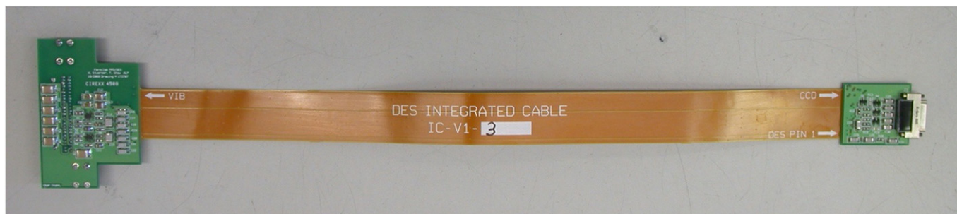
Figure 28. One of the Kapton cables that connects each CCD to the vacuum interface board. The JFET source follower is on the right. The video preamplifier is on the left. The connector for the preamplifier side is on the other side of the card.
