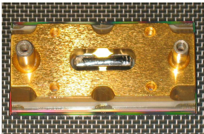
Figure 18. DECcam CCD shown with the illuminated back-side facing down. The CCD is at the bottom of the stack. Wirebonds in six places can be seen connecting the CCD to the aluminum nitride circuit. The gold-plated foot is at the top of the stack. The connector is shown in the center of the assembly. It has a shorting plug inserted in it for electrostatic protection. The two alignment pins are shown. Note that the one shown on the left has a larger diameter. That enforces orientation of the CCD on the focal plane. Also note the four small, threaded holes in the foot. These are for handling the CCD, particularly when the device is inserted into the focal plane.
