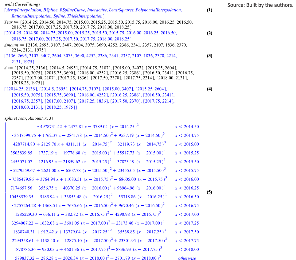
Figure 4. Practical realization of finding the predictive function by the method of splines extrapolation
