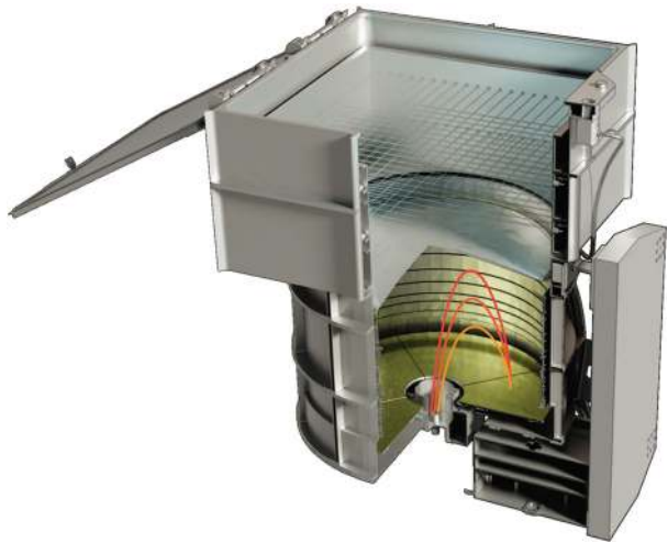
Fig. 14 Dust Telescope consisting of a trajectory sensor (on top) in combination with a large-area mass analyzer (below). In the cut-out ion paths (red) from the impact on the target to the central ion collector are visible (from the FOSSIL proposal, Horanyi et al. courtesy Tibor Balint, JPL)
