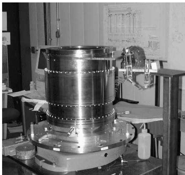
Figure 5. Final assembly of the camera on its rotating turntable.
