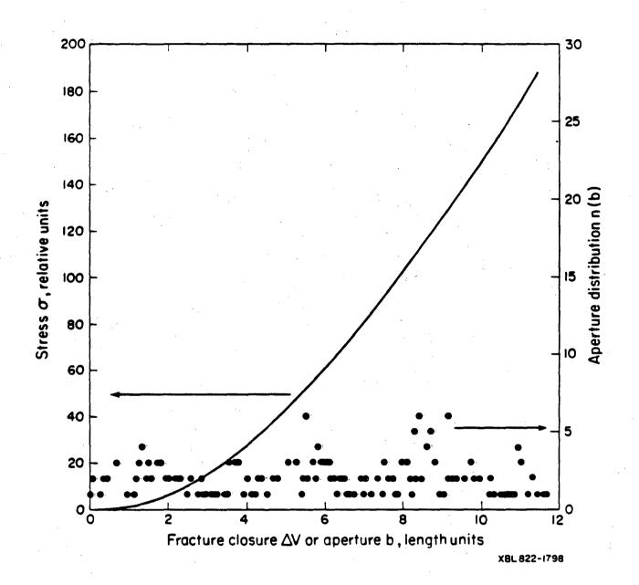
Figure 7. Fracture aperture distribution and stress-fracture closure variation for fracture 2d.
