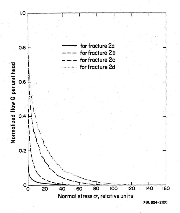
Figure 10. Normalized fluid flow per unit pressure head variation with applied normal stress for fractrures 2a-2d.
