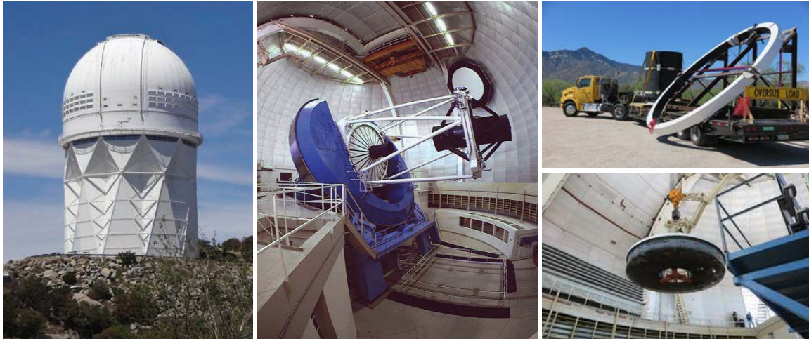
Figure 1. Shown on the left is the Mayall 4m telescope dome. The center image shows the telescope. The black cylinder is the MOSAIC corrector that will be replaced as part of the DESI project to instrument a 3 degree diameter field of view. The photos on the right show the new DESI prime focus cage and top ring arriving at the observatory. The Mayall primary mirror has already been removed to prepare for DESI installation
