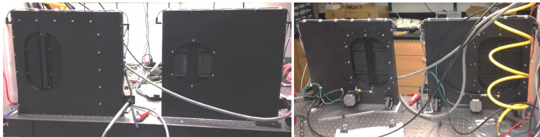
Figure 17: The shutter assemblies shown in the closed position with the exposure shutter on the left and the NIR shutter on the right. The views show the front (left) and reverse (right) sides of the shutters. The fiber illuminator LED is visible in the exposure shutter door front view. The motor and inflatable seal mechanism is visible in the reverse view.
