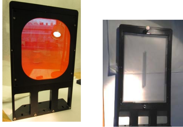
Figure 19: The mounts for the two dichroics. The one on the right has an uncoated substrate with a machined slot for fiber optic slit head to project light onto the collimator mirror.
