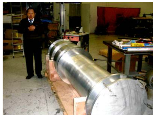
Fig. 1. The Magnet Forged 6061-T6 Mandrel during Machining.
