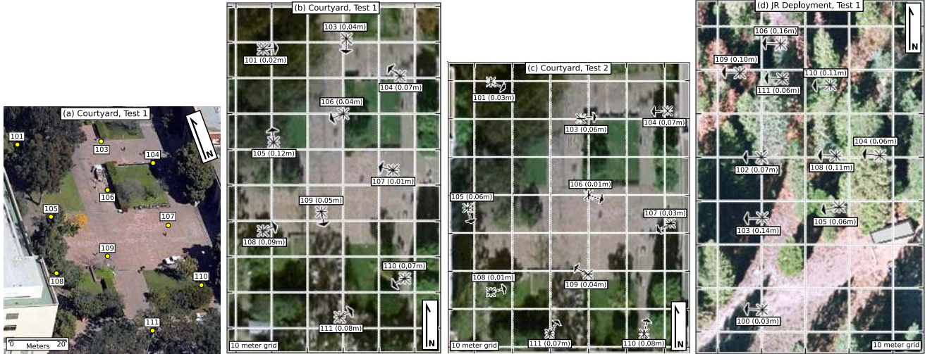
Figure 8. (a) shows a perspective view of the urban courtyard, with reflecting walls and tall, obstructing hedges and planters. (b), (c) and (d) show the experimental setup for our three test deployments: Courtyard 1, Courtyard 2, and the James Reserve in Idyllwild. Ground truth node locations are indicated by the X's. The '+' and arrow indicates a position and orientation estimate from our system, and the 2D position error in m is shown in parentheses. Photo credits: (a) Virtual Earth; (b) and (c) Google Earth; (d) the James Reserve.
