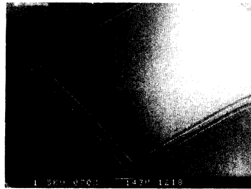
Fig. 6. SEM photograph of a square silicon nitride diaphragm with a square corrugation pattern.
