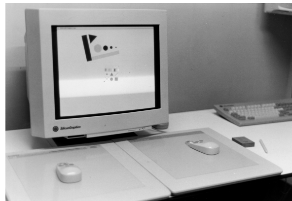
Figure 3: The input devices in T3. Two tablets with two rotation sensing pucks. A pen shown on the right can also be used instead of a puck. Just above the pen is a device called a "fip-frick."
