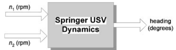
Fig. 7 Block diagram representation of a two-input USV
