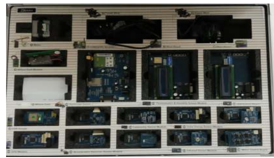
Figure 9: The Zigbee platform of the deployed WSN
