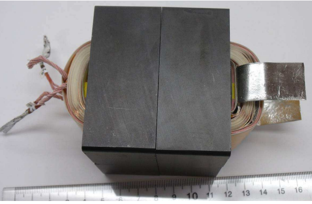
Fig. 2. Four-layer, interleaved foil winding prototype. The terminations of the secondary are on the right and the primary leads on the left.
