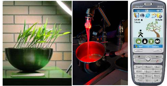
Figure 1. Examples of eco-feedback technology. (left-to-right) The Infotropism display uses sensors and living plants to provide feedback about recycling and waste disposal [29]. WaterBot provides ambient feedback information about water usage [3]. The UbiGreen Transportation Display semi-automatically senses and feeds back information about transportation to encourage green transit [19].
