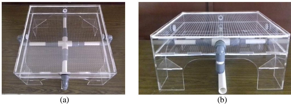
FIGURE 5. (a) Top view of 2D air track, (b) Side view of 2D air track
