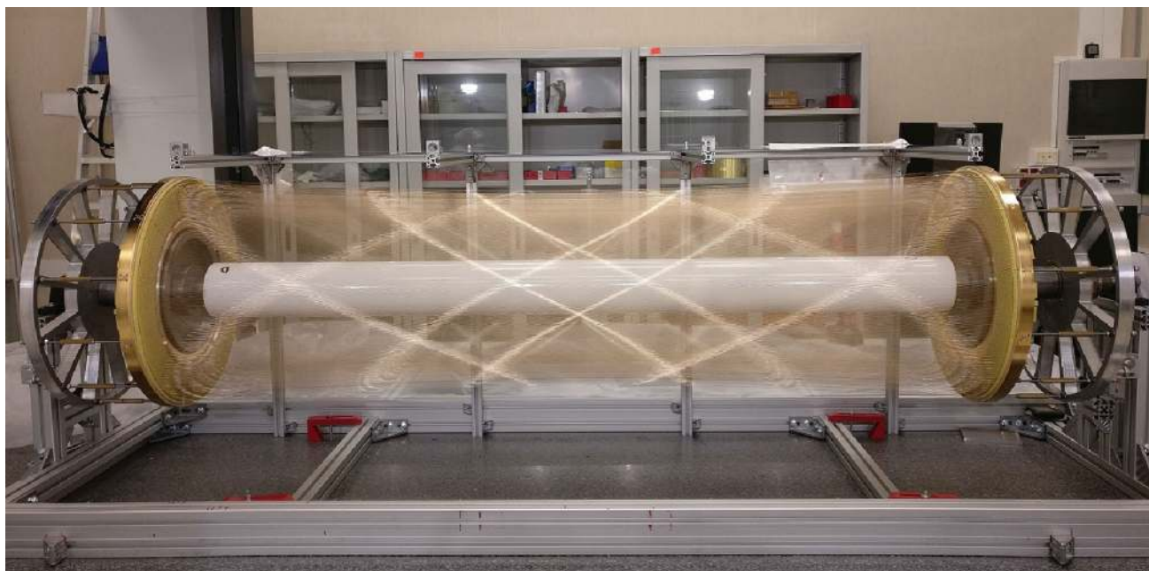
Fig. 33 The entire drift chamber with all layers mounted. The hyperbolic profile of the chamber is visible
