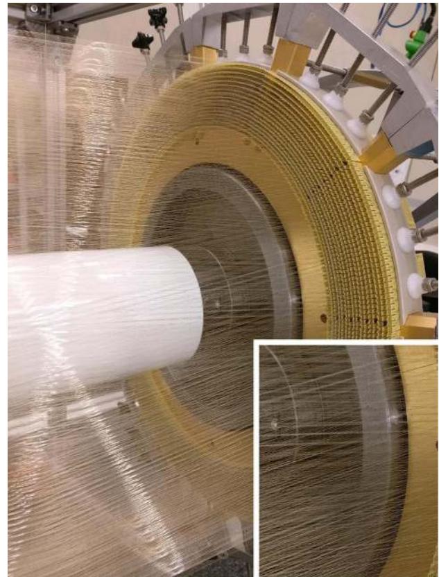
Fig. 32 A close view of an end-plate after assembling 80% of the layers, in the insert the crossing of the layers is shown
