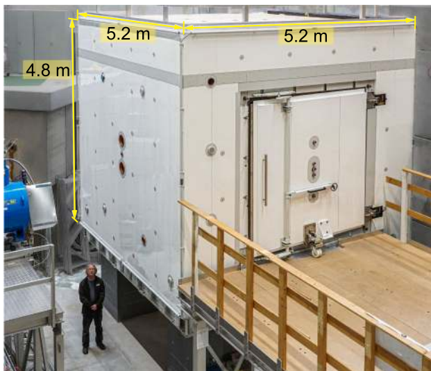
Fig. 19 Photo of the magnetically shielded room with indicated outer dimensions
