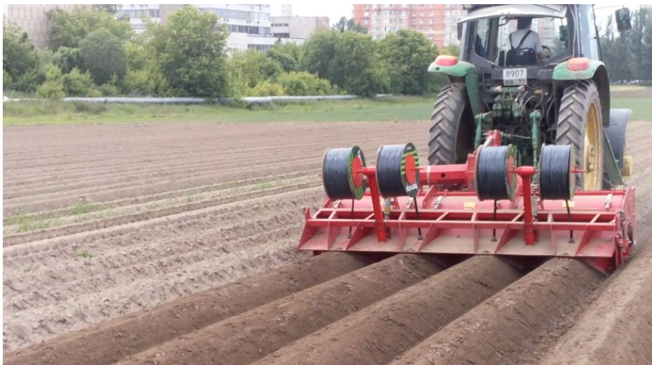
Fig. 4. Ridge-based drip tape stacker Grimme GF-75/4.
