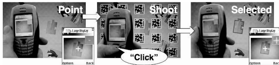
Figure 5. Summary of positioning techniques using a smart phone as an input device. © 1984, 2006 IEEE. Adapted by permission.
