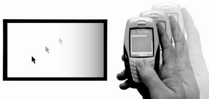
Figure 2. The Sweep technique uses camera input and optical flow image processing to control a cursor (Ballagas et al., 2005). © 2006 IEEE. Adapted with permission.
