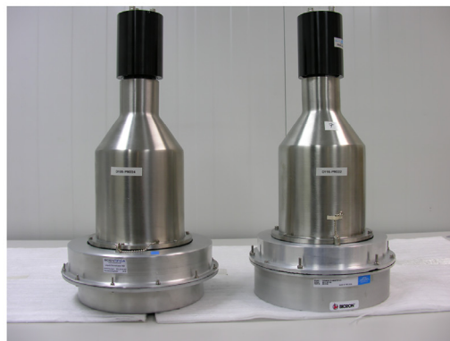
Fig. 11. Upper photograph: MONSTER array characterisation setup at Centro de Investigaciones Energéticas Medioambientales y Tecnológicas (CIEMAT). The detector cells are placed in the holding structure. Lower photograph: Two individual MONSTER detector cells.
