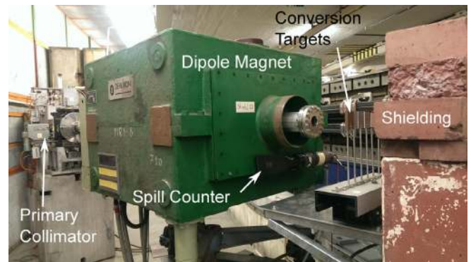
Fig. 6. (Color online) The test beam magnet (Type MR) of TB22. The secondary conversion target system is also visible in front of the magnets.
