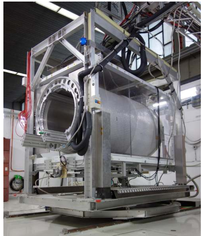
Fig. 20. (Color online) TB24/1 test beam area at DESY: movable lifting stage with the PCMAG 1 T solenoid.
