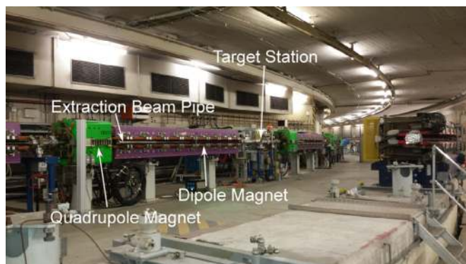
Fig. 2. (Color online) View of a section of DESY II on the left side of the DESY tunnel, the magnets on the right side are dipoles from the DESY III proton synchrotron.
