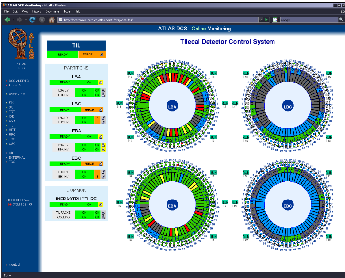
Figure 19. WWW monitoring page showing the online status of the Tilecal sub-detector.
