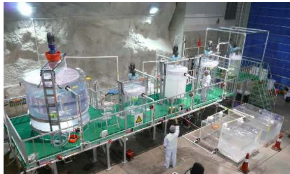
Figure 17: Prototype production system for the Daya Bay liquid scintillators. The upper diagram is of the prototype production system in IHEP. The lower photograph shows operation of the production system in the Daya Bay LS hall.
