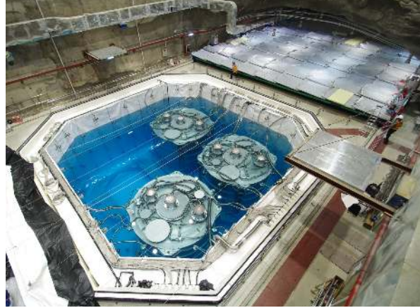
Figure 30: The partially filled far hall water pool containing three ADs is shown. Inner Water Shield (IWS) PMTs are visible above and below the water line. Outer Water Shield (OWS) PMTs are hidden beneath the white Tyvek TM sheets separating the IWS and OWS. Previously installed RPC arrays are rolled into the RPC garage area on the top-right to provide access to the water pool. Two sets of telescope RPCs are mounted on the hall walls as shown.
