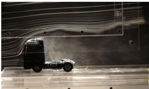
Fig.9. Flow visualization of truck
