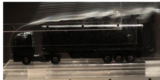
Fig.10. Flow visualization of truck and trailer
