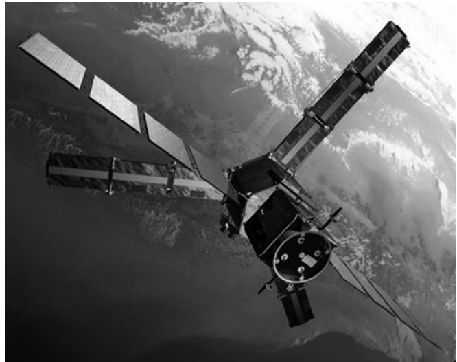
Fig. 1. (Left) Design of the Y-shaped MIRAS radiometer with 69 antenna elements (from EADS CASA Espacio). (Right) Artist's view of the SMOS spacecraft (from ESA Medialab).
