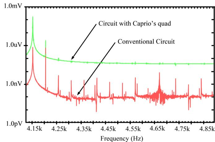
**Fig. 6.** Comparison of harmonic spectra of conventional circuit compared to Circuit with Caprio's quad
