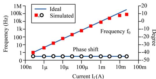
**Fig. 4.** Plot of the corner frequency (Hz) comparing the phase shift (degree) of  $V_O/V_{in}$  with versus the bias  $I_f$  (A) using a constant capacitance  $C = 10$  nF
