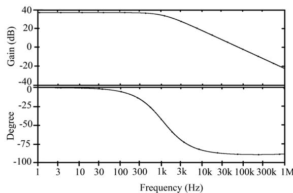
**Fig. 2.** The frequency response of  $V_O/V_{in}$  at room temperature with the  $I_T$  current set at 500  $\mu$ A and the capacitance  $C$  taken at 10 nF
