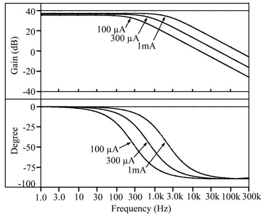
**Fig. 3.** Shows the magnitude (dB) and phase shift (degree) of  $V_O/V_{in}$  compared to the frequency (Hz) using capacitance  $C = 10$  nF and adjusted for current  $I_f = 100 \mu\text{A}$ ,  $300 \mu\text{A}$ ,  $1 \text{mA}$
