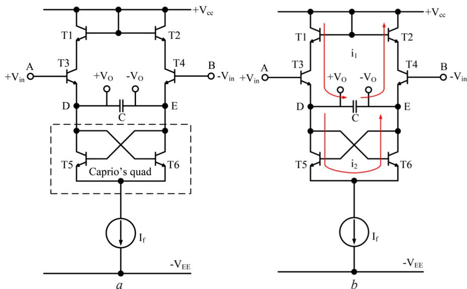
**Fig. 1.** A fully-balanced current tunable first-order low-pass filter with CAPRIO technique:
