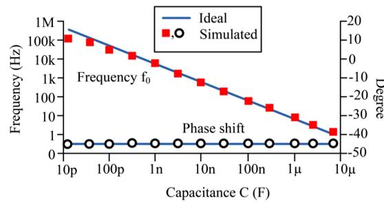
**Fig. 5.** Plot of the corner frequency (Hz) comparing the phase shift (degree) of  $V_O/V_{in}$  with versus the capacitance (C), using bias current  $I_f$  500  $\mu$ A
