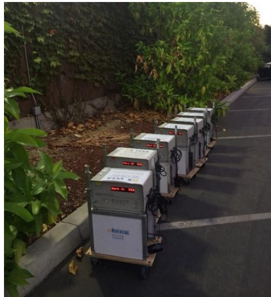
Figure 2-4- Co-location of CPCs before start of tests.
